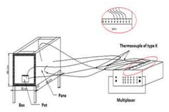
Figure 3 : Connexions between experimental device and data logger
